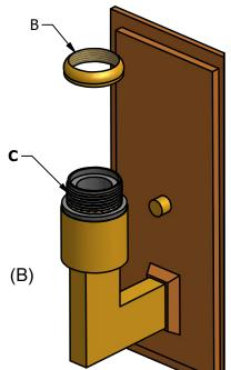
1. Unscrew the socket thread ring (B) from the socket (C).
