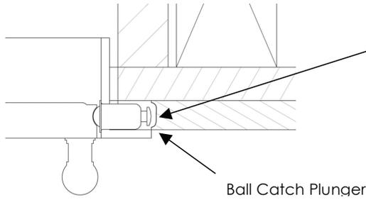
Note how ball catch plunger projects towards notch in the marble box when opening and closing the door. There must be clear space for this or else the frame may be damaged.
