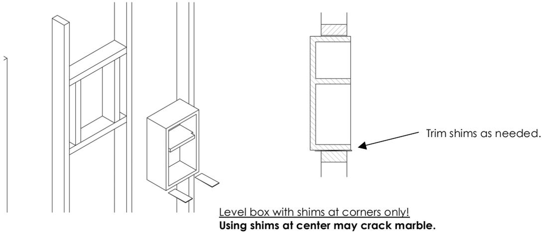
2. Install Backer Board flush with edge of framed opening. Backer board cutout dimensions are  $\frac{1}{4}$ " larger than the outside dimensions of the Marble Box.
