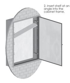
3. Rest shelf on the lower discs and secure with upper discs.
