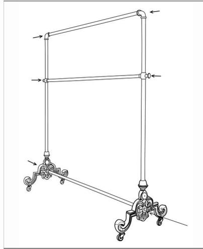
**STEP 5:** Tighten both Cap Nuts (part D), and all set screws.
