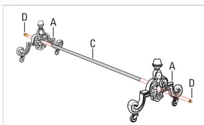
**STEP 1:** Place threaded rod from part C through hole in side of part A – loosely attach cap nut (part D) to outside end of threaded rod.
