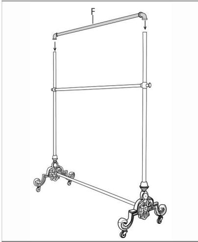
**STEP 4:** Insert decorative ends of Upper Cross Bar (part F) into top of two Upright Tubes (part B). Fix in place with provided set screws (short thread).
