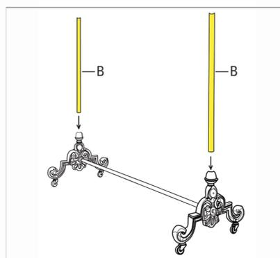
**STEP 2:** Insert Upright Tube (part B) into hole at top of foot (part A). Fix in place with provided set screw, long thread.
