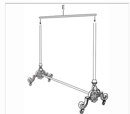
**STEP 3:** Open thumb screws on Middle Cross Bar (part E) so that holes are completely free of obstruction and gently slide Middle Cross Bar over both uprights at the same time, tighten thumb screws to hold in place.
