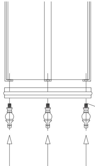
2. Slide the (C) base up over the arms. Screw (D) finials up into the base connecting it into the arms.
