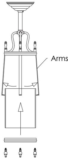
1. Flex the arms (A) slightly and slide the (B) glass cylinder, inside of the four arms.
