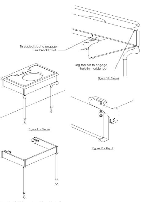
Figure 13 - Straight Leg version of the washstand has <u>Dimension E</u> = 0. The leg foot pin locations on the floor are the same as the pin hole locations in the marble top, <u>Dimensions C & D</u>.
