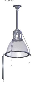
Close lens frame, rotate thread pin to a vertical position and secure in place with screw provided.
