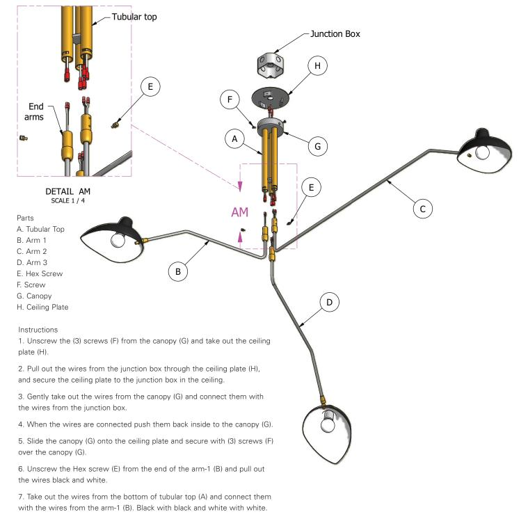
8. Push the connected wires inside of the tubular top and slide the end arm-1 (B) inside of the tubular top (A) and secure it with the Hex Screw (E).
