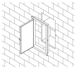
Install Silicone around the inside frame edge
