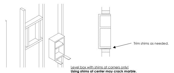
2. Install Backer Board flush with edge of framed opening. Backer board cutout dimensions are 1/4" larger than the outside dimensions of the Marble Box.
