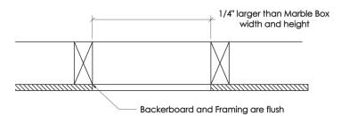
3. Set the Marble Box in the wall so that the front edge of box is flush with the backer board. Use construction adhesive that will provide 20 minutes of work time. Level the box with shims at the corners only. See sketch in Step 1.
