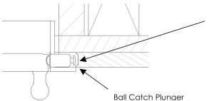
Note how ball catch plunger projects towards notch in the marble box when opening and closing the door. There must be clear space for this or else the frame may be damaged.
