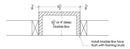
3. Install Drywall so that it covers the front edge of the Marble Box. Drywall cutout dimensions are the same as the interior dimensions of the Marble Box. The front edge of the box should not be visible.
