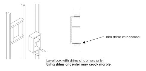
2. Set Marble Box in wall so front edge of box is flush with studded frame. Use construction adhesive to secure box in the frame. Use adhesive that will provide 20 minutes of work time.
