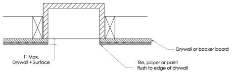
5. There is a ball-catch on the Lenox frame, which secures the door. For the catch to operate properly, a notch must be ground into the tile or drywall prior to frame installation. (See Fig 5.1) In order to mark the correct location for the notch, temporarily insert the Lenox Frame into the opening and mark the ball catch mechanism location. Clearance for the final shimming of the frame should be considered when positioning the notch. After marking the position, remove the Lenox frame.
