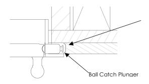
Note how ball catch plunger projects towards drywall / tile when opening and closing the door. There must be clear space for this or else the frame may be damaged.
