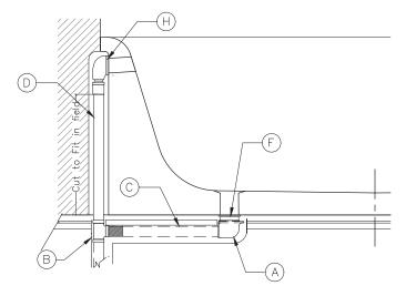
8. Screw the waste body and finish cover [G] into the spacer nut [F]
