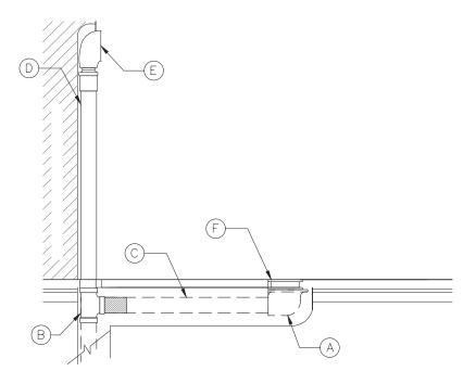
4. Screw the spacer nut [F] into the drain elbow [A]
